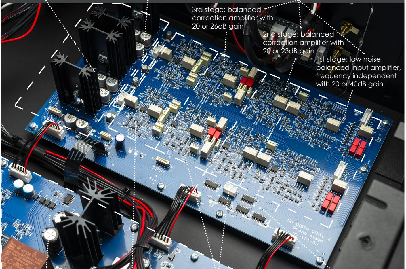
Separate discrete power filtering and DC blocking PCB
