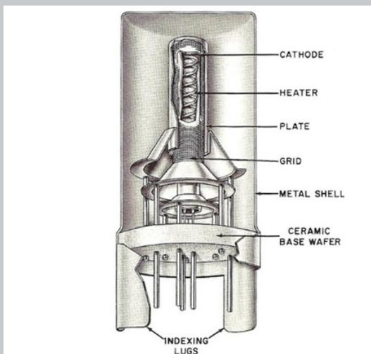
One famous application was in the Ampex MR-70, a costly studio tape recorder whose entire electronics section was based on nuvistors. Another limited application of this very small tube was in studio-grade microphones from that era, the AKG/Norelco C12a, which employed the 7586, being a good example.
